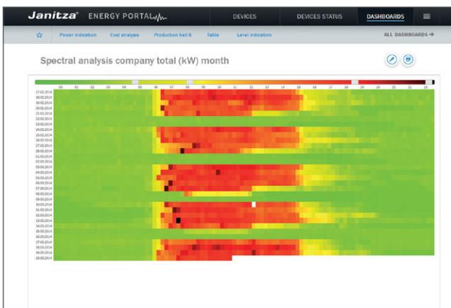
Heat map (spectral analysis) to determine peak loads that drive costs. The scroll bar in the chart's header area can be used to adjust the threshold values individually.
