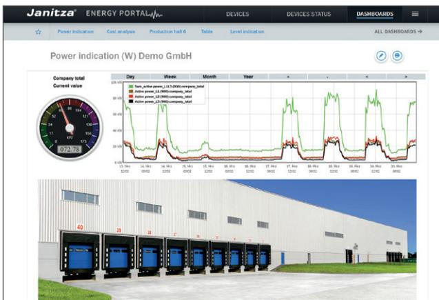
Example of a dashboard with a line chart (load profile) and the power value displayed using an analogue pointer display.
