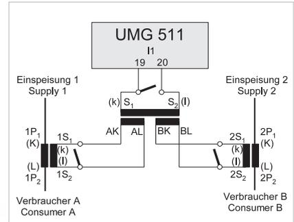
Fig.: Example, current measurement via a summation current transformer
